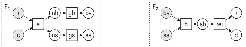
Figure 4.5. Two oclets F_1 and F_2 specifying behavior of the flood alert process of Sect. 2.1. Oclets do not require to assign each event to a specific component.
