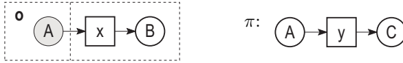
Figure 4.18. The run \pi respects progress of oclet o , but \{\pi\} is not closed under continuations with o .
