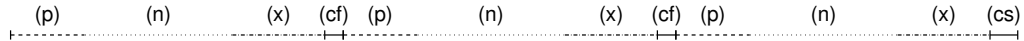
Fig. 5. Accumulated delay after three cognate arrivals: (p) delay (f_p/f_c) \cdot T_f^p for failing pseudo-cognates, (n) delay (f_n/f_c) \cdot T_f^n for failing near-cognates, (x) delay (f_x/f_c) \cdot T_f^x for non-cognates, (cf) exit time T_f^c for a failing cognate, (cs) exit time T_s^c for a successful cognate.
