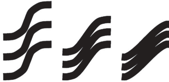
Figure 5. Sharp-angle, straight-limb folds give rise to smaller void spaces than rounded folds.
