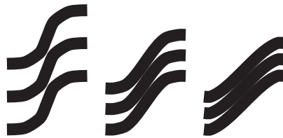
FIG. 10. Sharp-angle, straight-limb folds give rise to fewer voids than rounded folds (after [8]).
