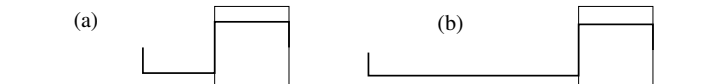
Fig. 3. A symmetric wavelet analysis (bold line) is not optimal in detecting change points. If one allows unbalanced analyzes, the resulting wavelet coefficients may be more significant if the analysis covers two complete, adjacent intervals of constant intensity. This may be crucial in change points with small jumps.
