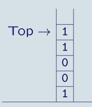
Besides the input symbol and current state, also the symbol at the top of the stack determines which transition the PDA takes.
