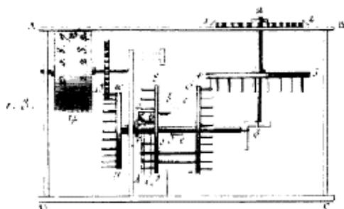
**Figure 5: The connection between the carry mechanism and the discs at the top of the pascaline**
