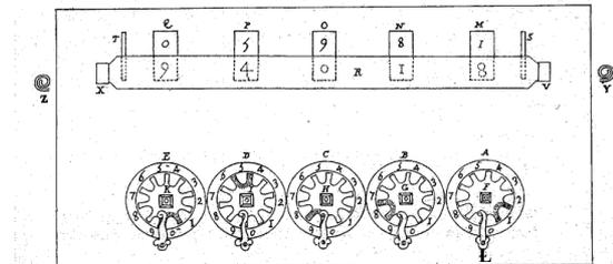
Figure 2: Schematical representation of the top of the pascaline
