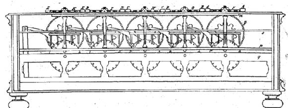
**Figure 4: A sideview of the pascaline. We see the carry mechanism repeated at each wheel**
