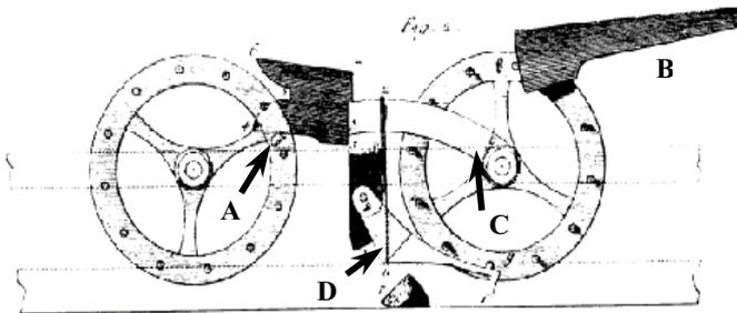
**Figure 3: The carry-mechanism of the pascaline, seen from the side**
