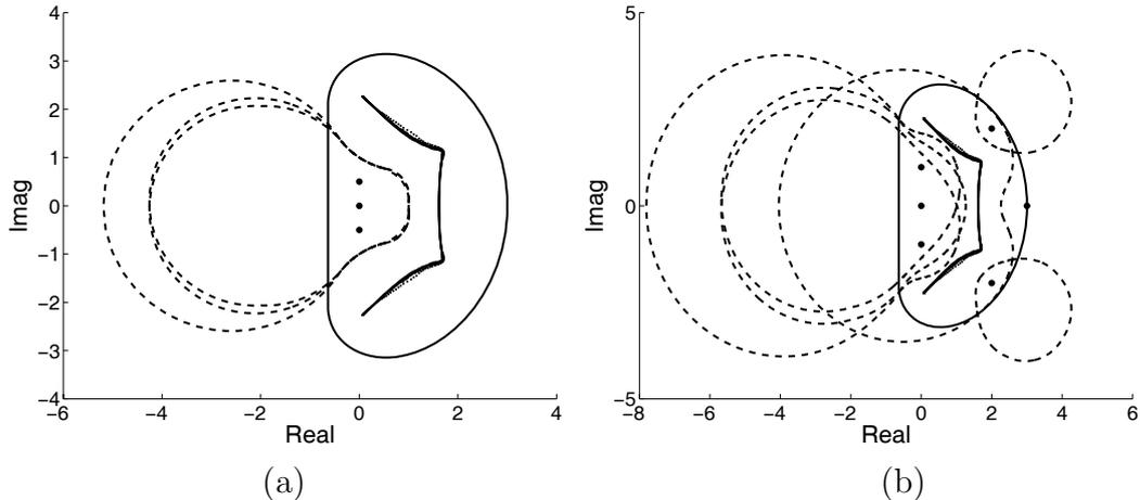
Fig. 3. (a) Spectrum,  $W(A)$  (solid) and  $1/W((A - \tau I)^{-1}) + \tau$  (dotted) of the  $1000 \times 1000$  `grcar` matrix and targets  $\tau = 0, \pm i/2$ . The targets are indicated by an asterisk. (b) The same but here the sets  $1/W((A - \tau I)^{-1}) + \tau$  (dot) are numerically *approximated* by (12) using a 10-dimensional Krylov space. We use the targets  $\tau = 0, \pm i, 2 \pm 2i$  and 3.
