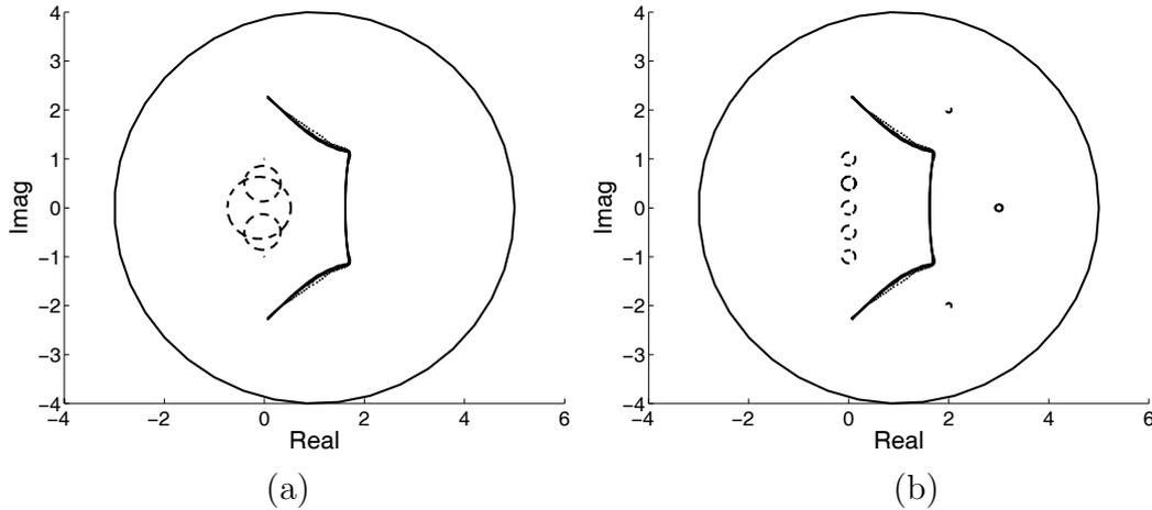
Fig. 4. (a) Spectrum,  $\Gamma(A)$  (solid) and  $1/\Gamma((A - \tau I)^{-1}) + \tau$  (dot) of the  $1000 \times 1000$  `grcar` matrix for shifts  $\tau = 0, \pm i/2, \pm i$ . Note that the exclusion regions for  $\tau = \pm i$  are so tiny that they are hardly visible. (b) Spectrum,  $\Gamma(A)$  (solid), and Krylov approximations to  $1/\Gamma((A - \tau I)^{-1}) + \tau$  (dotted) for several values  $\tau = 0, \pm i/2, \pm i, 2 \pm 2i$ , and 3.
