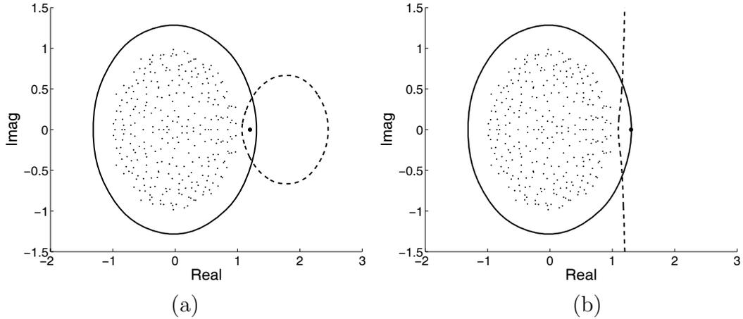
Fig. 1. (a) Spectrum,  $W(A)$  (solid) and  $1/W((A - \tau I)^{-1}) + \tau$  (dot) of the  $300 \times 300$  `randcolu` matrix for the shift  $\tau = 1.2$ , also indicated by an asterisk. The dotted line is the boundary of the unbounded inclusion region  $1/W((A - \tau I)^{-1}) + \tau$  and its bounded complement which forms an exclusion region. (b) Idem but now for  $\tau = 1.3$ , which is still inside  $W(A)$ . As a consequence, the inclusion region is therefore still unbounded.
