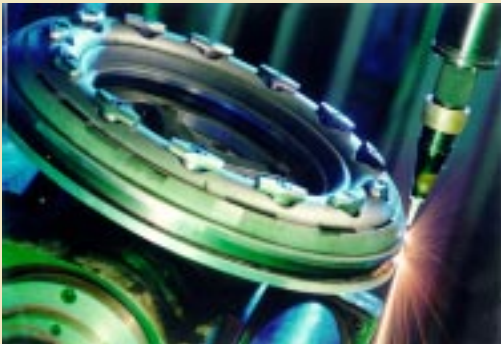
Figure 1 : A photo of a laser percussion drilling process in action. (By permission of ELDIM B.V.)
