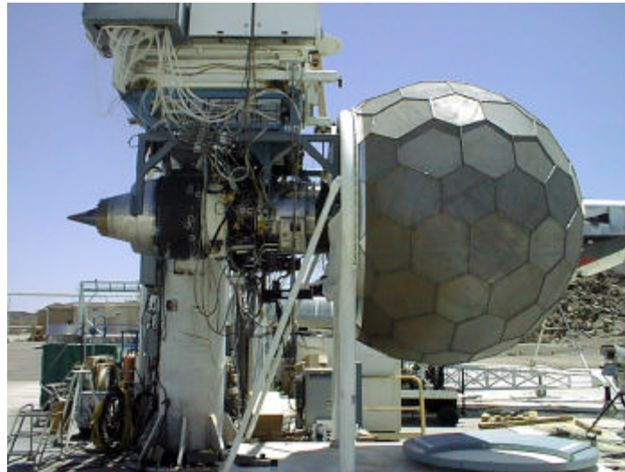
TFE731-60 Engine with Inflow Control Device (ICD)
