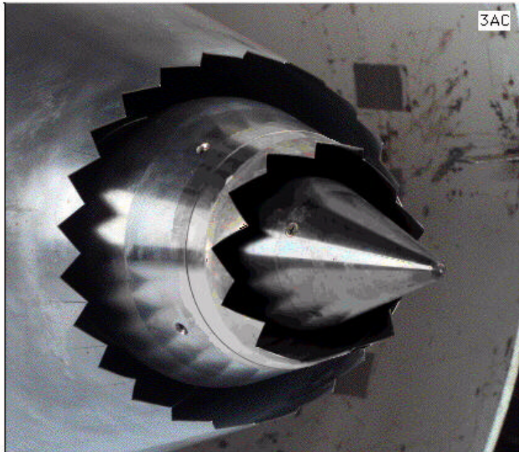
Fan Chevrons with Core Alternating Chevrons
