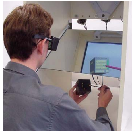
Figure 1. The user manipulates two interaction devices (pen and cube) in order to control the corresponding virtual objects (displayed in the PSS). The stereo cameras with infrared light sources are (partly) visible in the back.
