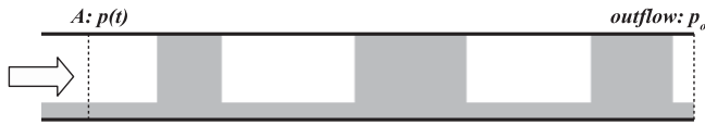
Fig. 5. Example of the slug length and film length in piping downstream of the bend.
