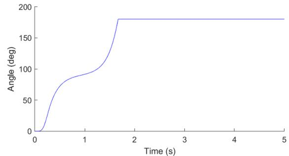
FIGURE 23. Cover angle in degrees,  $v_{in} = 24.5$  m/s
