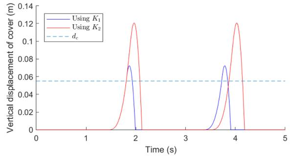
FIGURE 5. Cover displacement,  $v_{in} = 1 \text{ m/s}$
