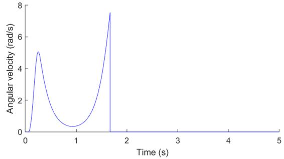
FIGURE 22. Angular velocity of the cover,  $v_{in} = 24.5$  m/s
