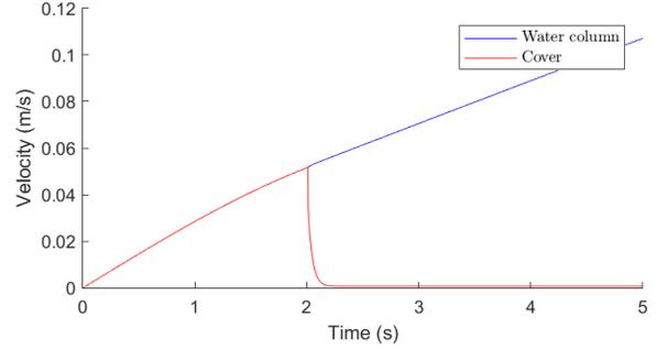
**FIGURE 13.** Water column and cover velocities,  $P_{in} = 5.96$  bar
