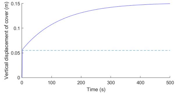
**FIGURE 15.** Cover displacement over 500 seconds,  $P_{in} = 5.96$  bar
