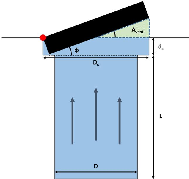
FIGURE 2. Manhole cover rotated around a hinge
