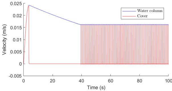
FIGURE 16. Water column and cover velocities,  $P_{in} = 5.9505$  bar
