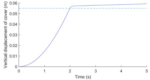
**FIGURE 14.** Cover displacement over 5 seconds,  $P_{in} = 5.96$  bar
