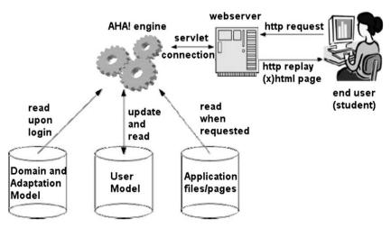
Fig. 1. AHA! architecture and data stores used by the AHA! engine.
