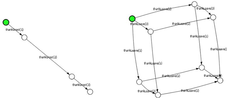
Labeled transition system for the specification of Appendix A with only actions **showTicket** and **clarify** by the **Client** processes shown. It validates that all three clients can raise their ticket independently, since admitted local behavior can be executed asynchronously from other component behavior, but are served in order of their ticket.
