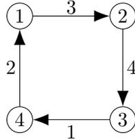
Then we have a deadlock: every channel wants to switch to a next channel since the destination is different from the target of the channel. But this is blocked for every channel since every next channel is occupied. As every node has exactly one outgoing channel, there is no choice in defining *route*.
