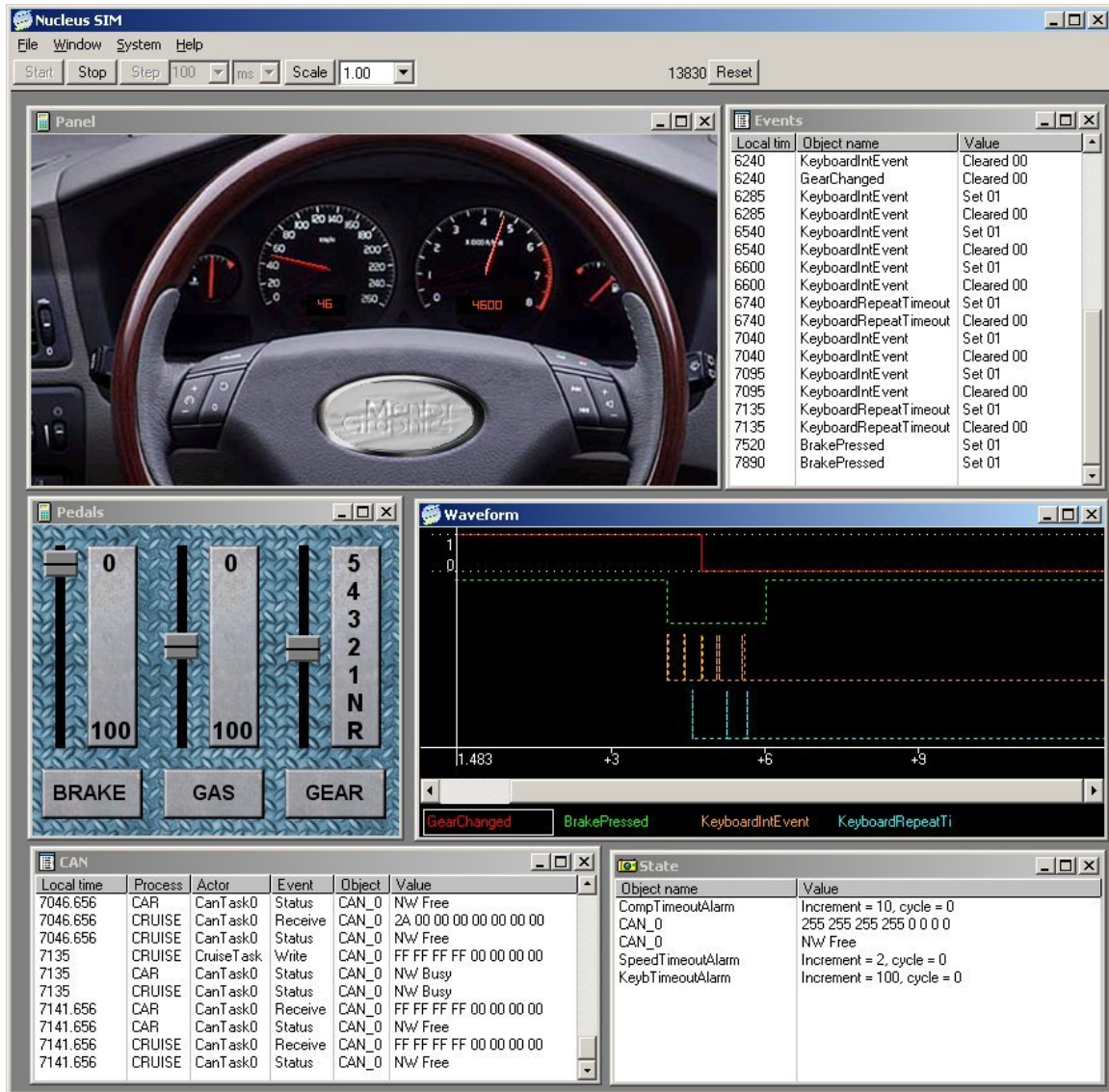
Figure 1: A system simulation environment for automotive software
