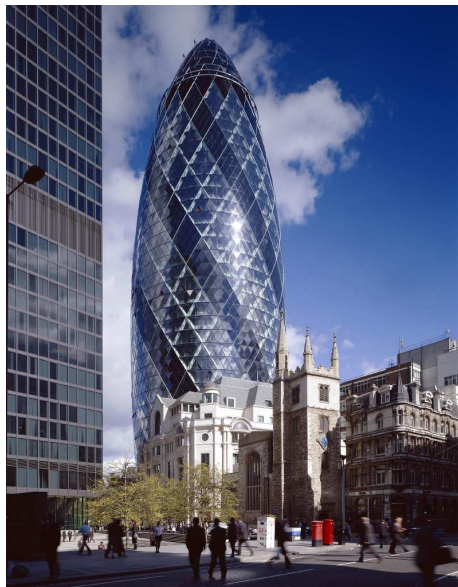
Figure 1.5: The Gherkin in London (Photo Nigel Young/Foster and Partners). Rotating the point (x, f(x), 0) around the x -axis (right). For each value of x this produces a circle with equation y^2 + z^2 = f(x)^2 . Apart from details, the shape of the gherkin comes close to a surface of revolution.
