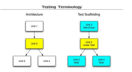
Test case: control activation and input; observe response and output; decide on pass/fail. 13
