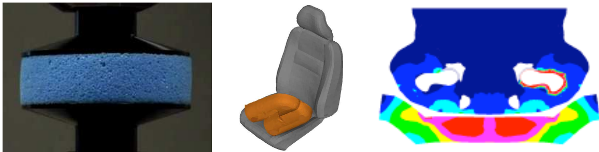
Figure 1: Experimental setup of foam testing, typical application of foam, simulation results
