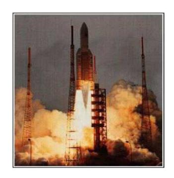
The launcher began to disintegrate at about 39 seconds because of high aerodynamic loads resulting from an angle of attack of more than 20 degrees.
