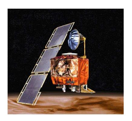
Cause: unchecked type mismatch of metric and imperial units
