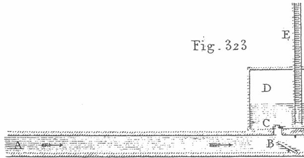
**Figure 3** The hydraulic ram of Montgolfier (15, Vol. 2, Fig. 323). When the water in the pipe AB has acquired a sufficient velocity, it raises the valve B, which stops its passage, so that a part of it is forced through the valve C, into the air vessel D, whence it rises through the pipe E.
