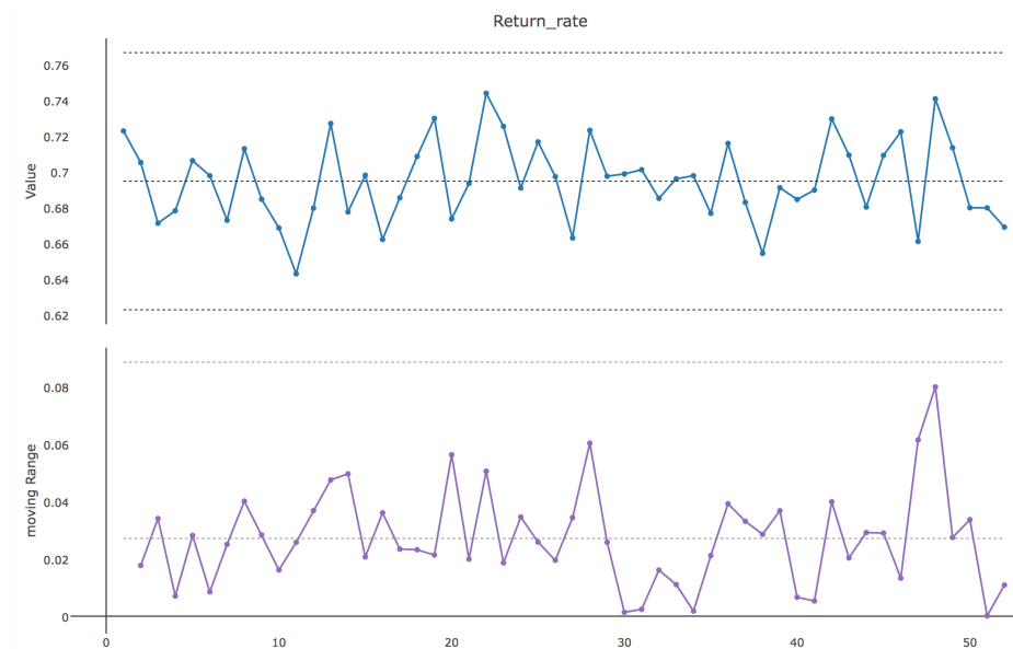
Fig. 20. XmR-chart for the return-rate: all common-cause variation
