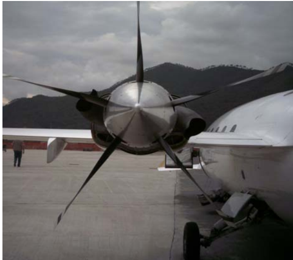
Figure 4.4: P180 Ground noise test for exhaust shape and orientation optimization
