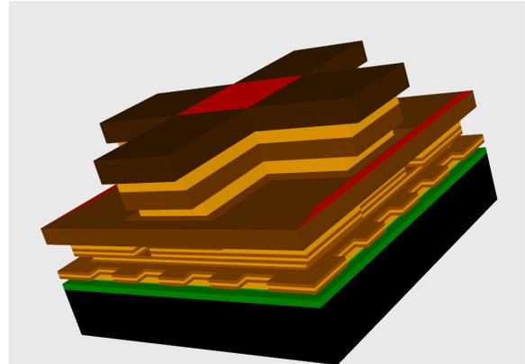
Fig. 1: 3D view of the ESD protection device.
