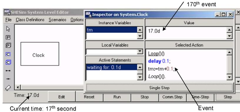
Figure 6: A clock model in SHEsim
