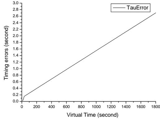
Figure 2: Accumulated timing errors of a TAU 2 clock implementation
