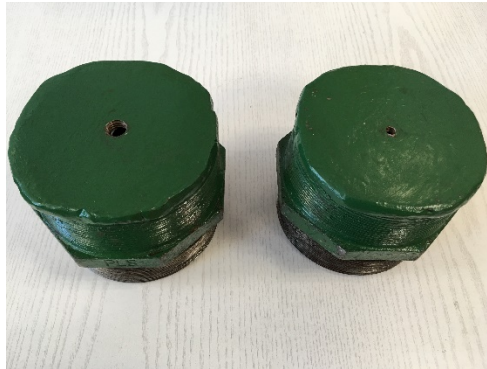
Figure 11. Orifice plates (end caps) with D_0 = 10 mm (left) and 5 mm (right) diameters
