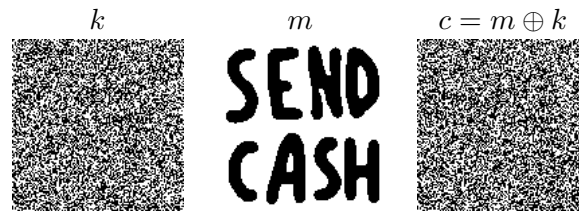
Figure 4.171: A 128 \times 128 -image encrypted by a random one-time pad key: white is 0, black is 1
