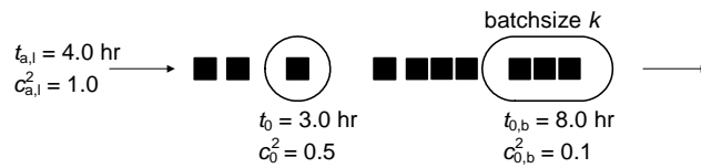
Figure 3.9: Single-lot machine and batch machine in series
