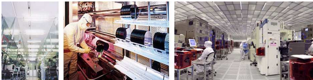
Figure 10.7: (a) Furnace bay (source: Micron Technologies), (b) Single (horizontal) furnace (source: Micron Technologies), and (c) Lithographic area (source: Crolles2 waferfab)
