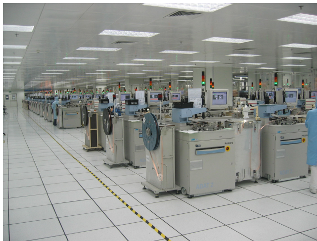
Figure 4.3: BIM (Breakthrough in Manufacturing) lines of NXP for the assembly of ICs
