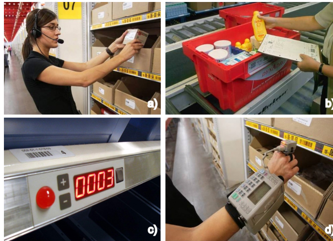
Figure 1.7: Four interface types: Pick-by-voice (a), Paper based picking (b), Pick-to-light (c) and a RF-terminal (d)
