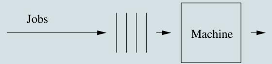
A single machine processes jobs in order of arrival. The interarrival times and processing times are exponential with parameters  $\lambda$  and  $\mu$  (with  $\lambda < \mu$ ).
