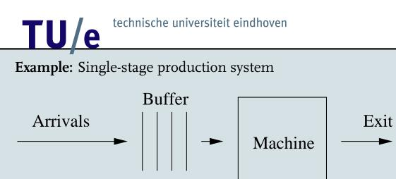
A single machine processes jobs in order of arrival. The interarrival times and processing times are exponential with parameters  $\lambda$  and  $\mu$  (with  $\lambda < \mu$ ).
