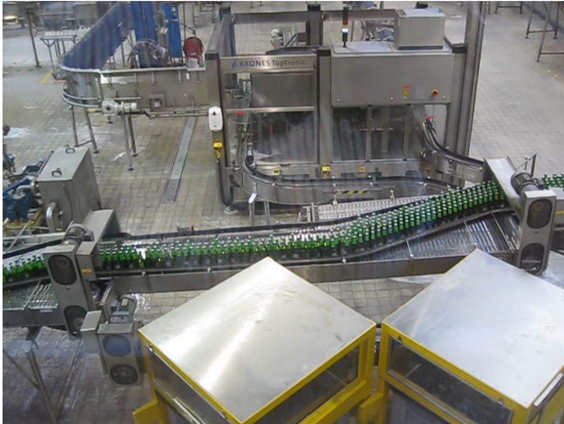
Conveyor system: transportation and buffering
