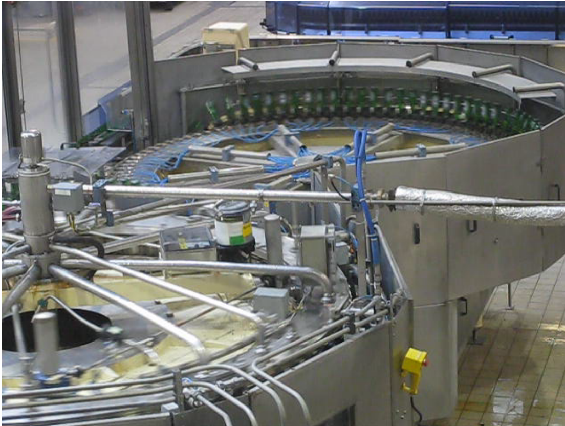
The filler: a carrousel filling bottles at high speed
