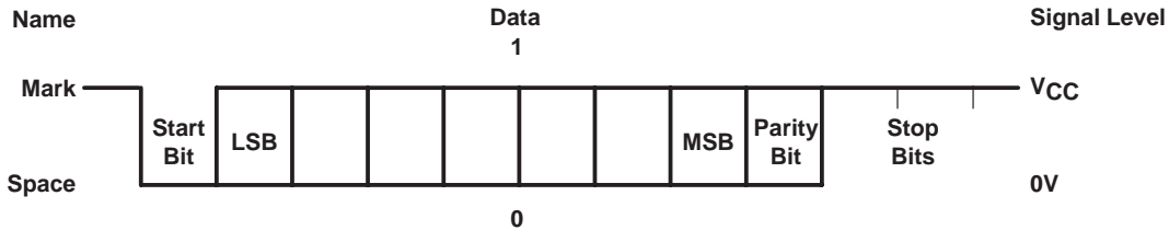
Figure 3. RS232 Format (Levels at the MSP430)
