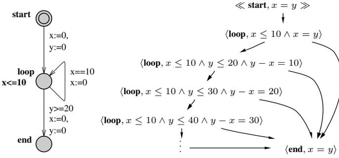
Fig. 4. A Timed Automaton with an Infinite Zone-Graph.
