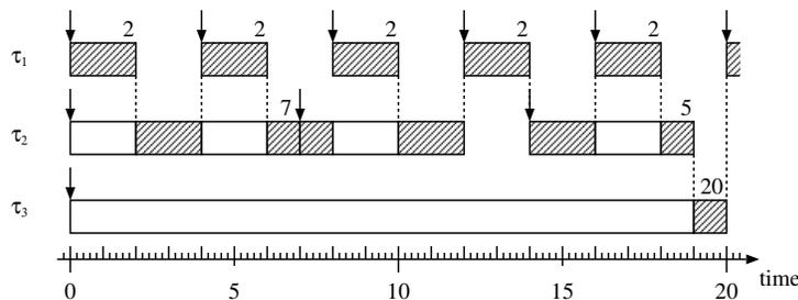
Figure 1: Time line with a critical instant for task  $\tau_3$ .
