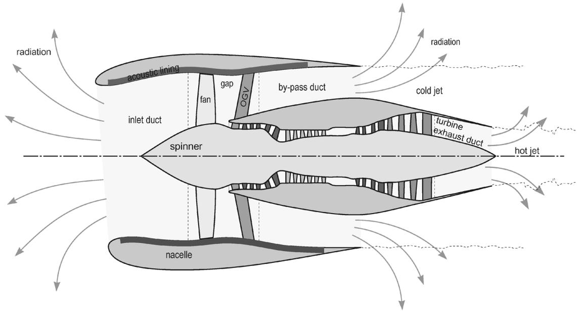
Fig. 1 Zones in a typical high-bypass-ratio turbofan engine.
