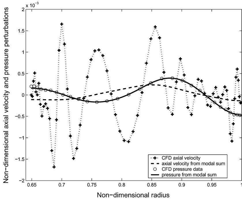
Fig. 6 Bypass fan/OGV test case; axial velocity and pressure perturbations obtained from the TPP matching and reconstructed using the homentropic potential flow model vs original CFD data at  $x = 0.344$  m.
