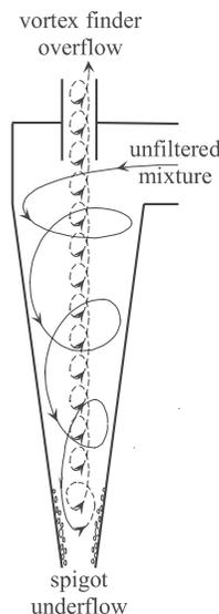
Figure 2. Schematic of a conical separator depicting its key components.
