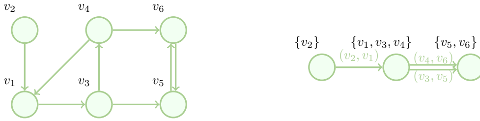
Figure 6.2: The graph on the right shows visualisation of the effect of the function \text{condense}(G) , on the graph on the left
