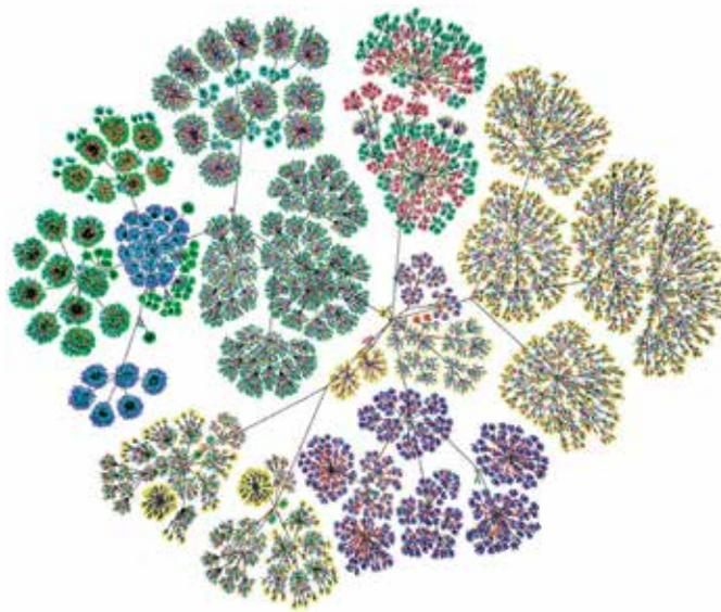
An illustration of the communication hierarchy in the control software. Each small software component is one of the coloured dots in the figure, and the lines between two dots indicate that the components they represent are connected and communicate directly with one another. Same-coloured nodes in the figure indicate that the components run the same software programs, whereas different coloured nodes run different programs.
