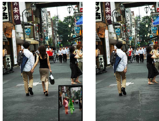
Figure 11: Simple object removal: the user marks a region for removal (green), and possibly a region to protect (red), on the original image (see inset in left image). On the right image, consecutive vertical seam were removed until no 'green' pixels were left.
