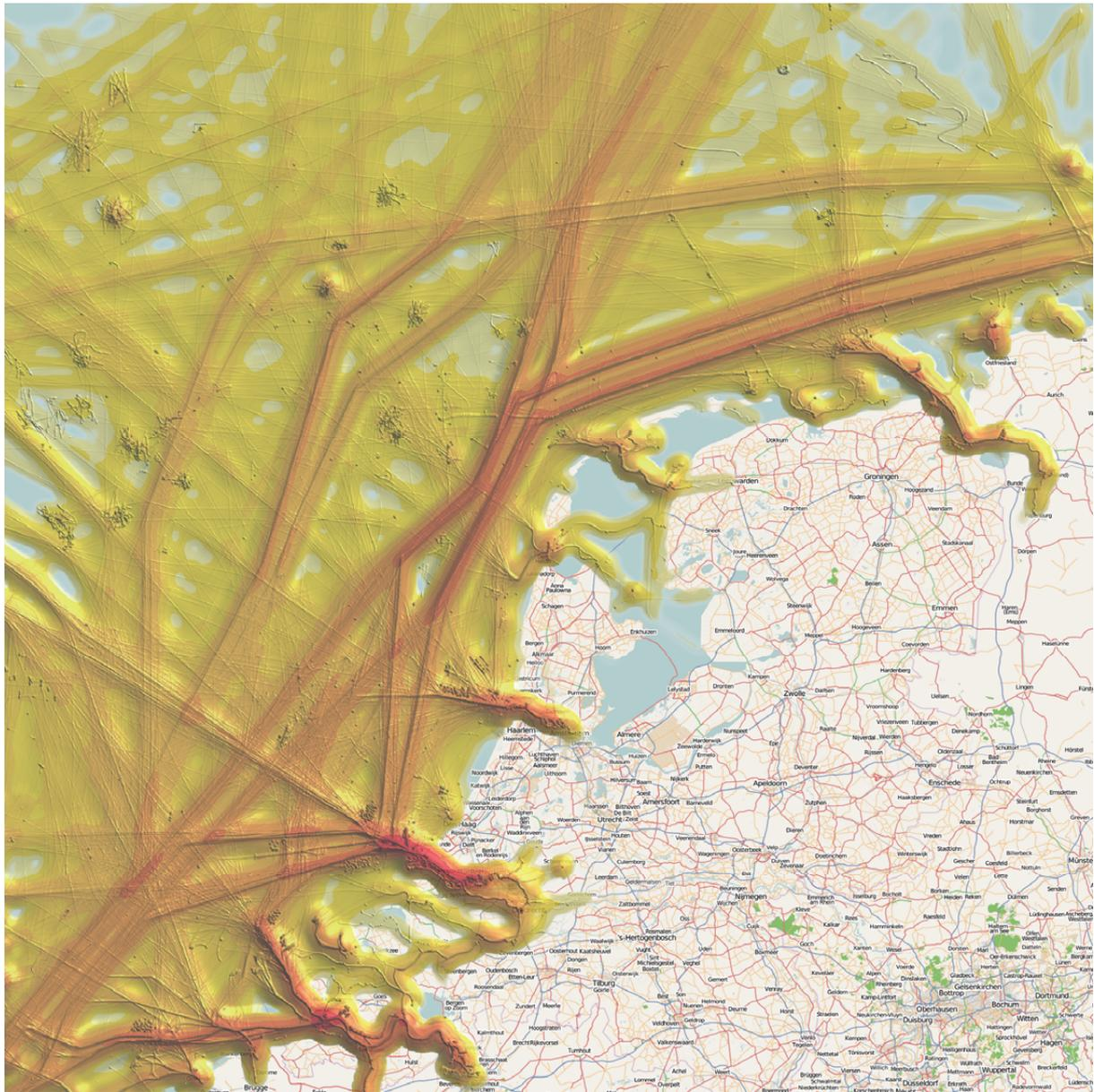
Figure 1: Vessel density in front of the Dutch coast
